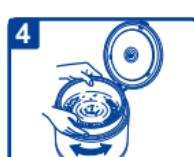
Be sure to wipe dry the outside of the pan. Then place the pan into the body and turn it slightly right and left until it seats properly.
