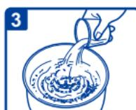
Fill the pan with water. Markings inside the pan show required amounts of water. E.g.: If you use two cups of rice, fill the pan with water until the line marked 2, or use the table below for your reference. You may adjust the composition between water and rice to your preference.
